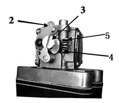
风门, 冷启动时使用; Choke Arm (The Choke Arm is used under the circumstance of cold start-up.); (2)、油门; Throttle; (3)、怠速调节螺丝; Idle Adjustment Screw; (4)、低速油针; Low-speed Needle; (5)、高速油针; High-speed Needle;
